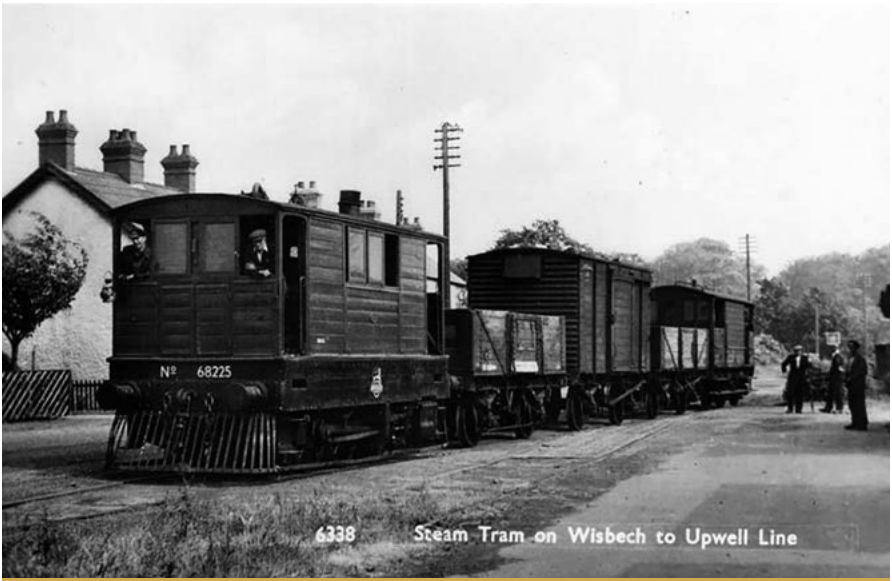
Steam Tram, Upwell. This steam tram was a J70 0-6-0, originally the GER Class 53. Postcard from the author's collection.
